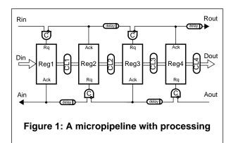
data comes to the micropipeline from outside and is transferred through the stage registers. If there are no processing blocks (usually combinational circuits) between stages the micropipeline performs as an ordinary first-in first-out (FIFO) buffer. The data processing procedure is controlled by C-elements which are state-holding 'rendezvous' elements performing the AND function for events.
