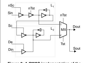
Figure 2: A CMOS implementation of the scan latch
