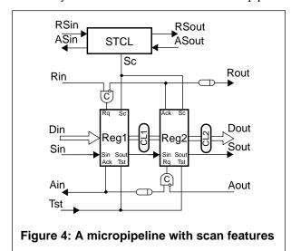
It also generates shift clock signals *Sc* for a united shift register. The STCL block can serve either a 2-phase or 4-phase signalling protocol depending on its structure. The STCL can either be a central control block or can be incorporated inside some of the micropipeline registers. Similar STCL units can be used in different parts of the chip to arrange an asynchronous scan test control interface between different asynchronous blocks.
