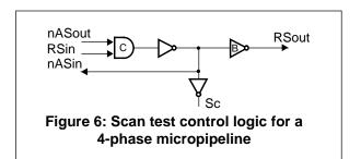
goes high and a rising event is generated on the request output *RSout*. If *nASout=RSin*=0 the C-element is set to zero. Thus, the signal *Sc* is reset to zero, rising and falling events are produced on the control lines *nASin* and *RSout* respectively. The delays of the control signals in the STCL block are presented in Table III. The results show that the use of the 4-phase STCL block improves the performance of the shift operation.
