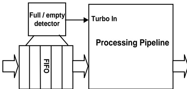
Figure 10. Controlling the Turbo Input According to Demand
