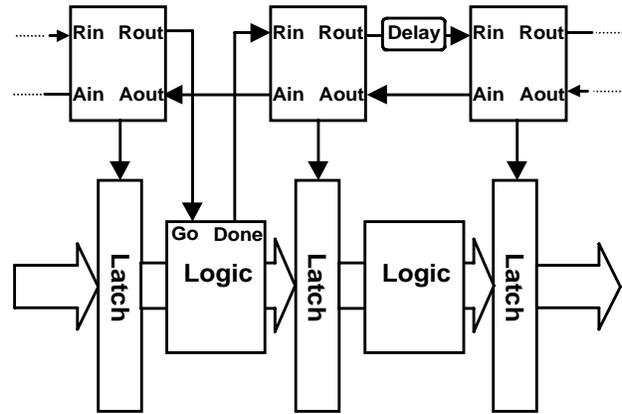
**Figure 2. Asynchronous Pipeline with Processing**
