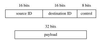
Here the 8-bit control field includes packet type (=1 for p2p packets), a data payload indicator, a sequence code, time stamp and error detection (parity) information, plus a spare bit for software
