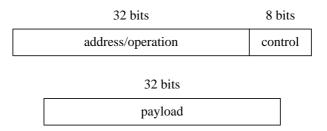
Here the 8-bit control field includes packet type (= 10 for nn packets), routing information, a data payload indicator and error detection (parity) information:
