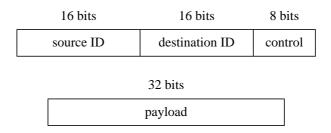
Here the 8-bit control field includes packet type (=01 for p2p packets), a sequence code, time
