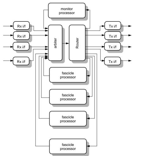
Each chip contains 20 identical processing subsystems each of which is responsible for modelling a number of neurons with associated inputs and outputs - a fascicle.
