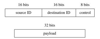
Here the 8-bit control field includes packet type (=01 for p2p packets), a sequence code, time
