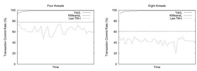
Fig. 2. Sample observed transaction commit percentages (using the Priority CM). VacL has far more commits (i.e., less contention) than Lee-TM-t or KMeansL
