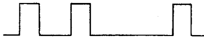
Fig. 1. Representation of binary digits by presence or absence of pulses. The binary number 1101 is equivalent to 2^3 + 2^2 + 0 + 1 , i.e., 13 in decimal notation
