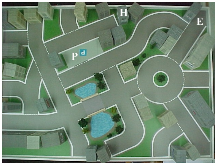
Figure 2. Miniature town in which a robot will navigate according to route instructions given by users.
