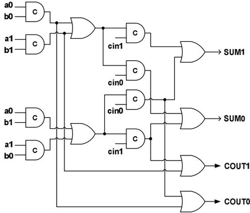
Figure 8. Folco et al.'s weak-indication full adder
