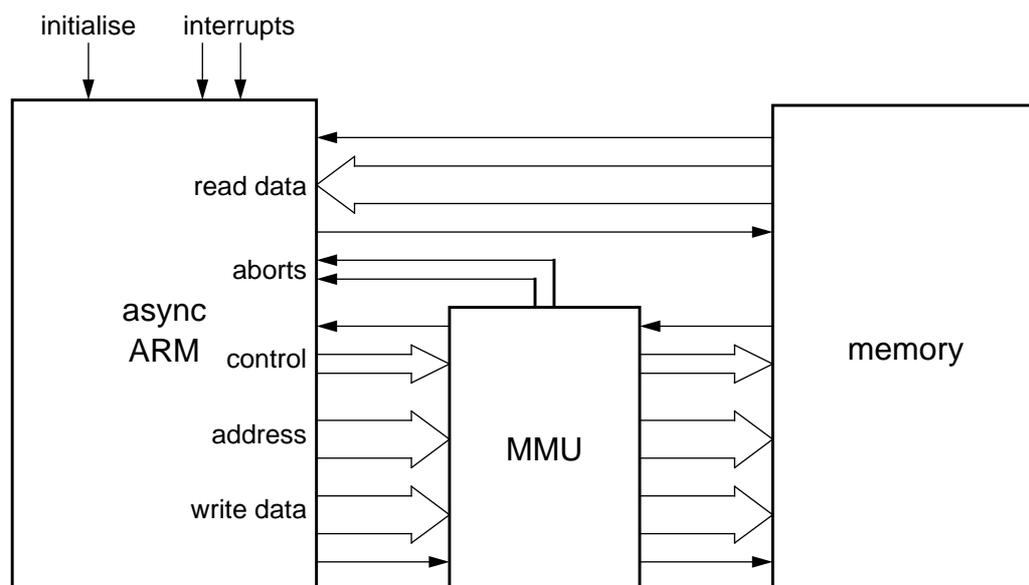
Figure 2. The processor interface
