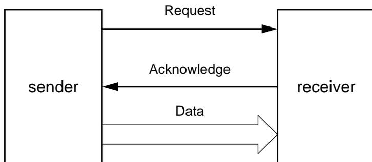
Figure 1. A two-phase bundled data interface
