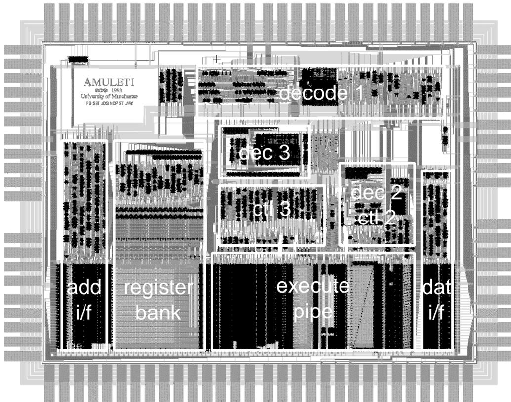
Figure 10. The asynchronous ARM chip
