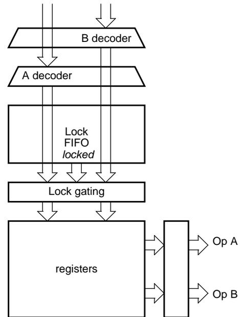
Figure 7. The register read logic
