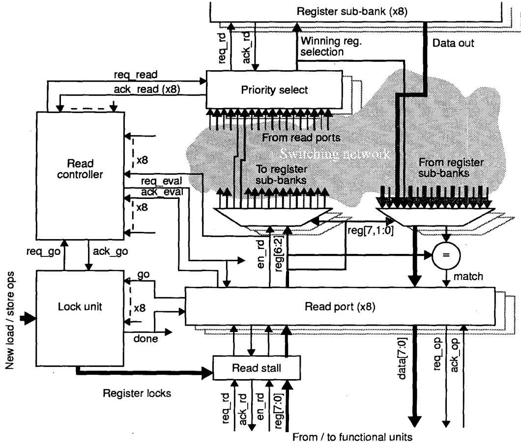
**Figure 7 Read mechanism**
