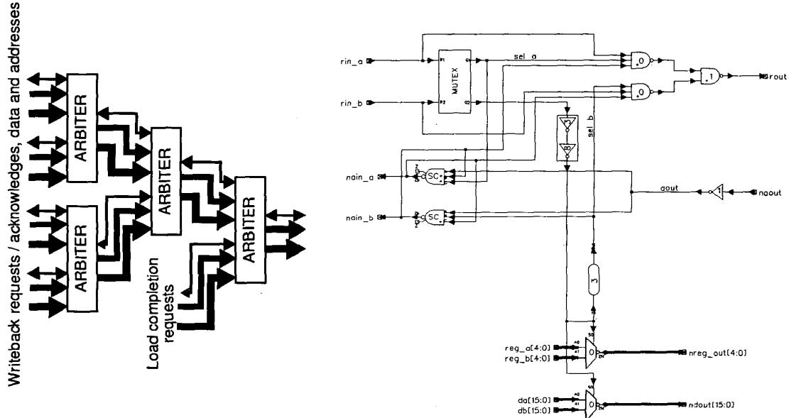
**Figure 6 Arbitration block structure and arbitration component**
