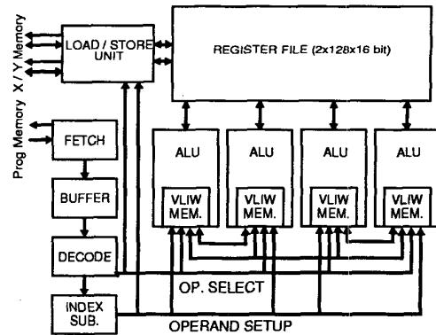
Figure 1 Block Diagram of CADRE
