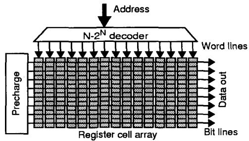
Figure 3 Word and bit lines in a register bank
