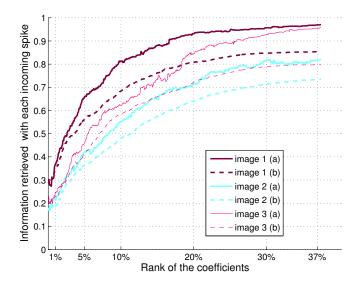
**Figure 7.** Information recovered from three different rank-order encoded images using the two methods of reconstruction viz. (a) pseudo-inverse of the DoG filter-bank and (b) the DoG as its own inverse.
