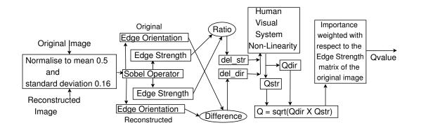
Figure 3. Flowchart of Petrovic's algorithm as used in our work
