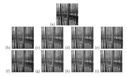
Figure 2. (a) input image (b)–(e) Reconstructed image using 1%, 5%, 10% and 20% respectively of the coefficients of filtering with the DoG. (f)–(i) Reconstructing rank-order encoded image using the first 1%, 5%, 10% and 20% of the values respectively from the LUT.
