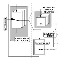
Fig. 12. An event-driven framework. The left side is the model space, consisting of callback routines. The right side is the system space, consisting of a scheduler and interrupt-service routines.
