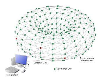
Fig. 2. SpiNNaker system topology.
