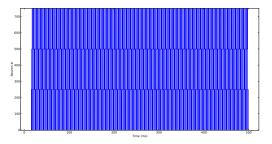
Fig. 9. Simulation of a highly synchronous synfire chain model. The system simulates 3 populations of 300 neurons each. All neurons fire in precise synchrony - a worst-case test for the packet-handling system
