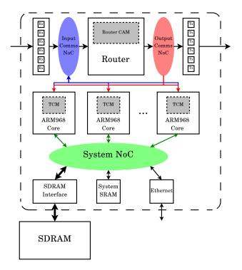
Fig. 3. SpiNNaker Architecture. The dashed box indicates the extent of the SpiNNaker chip. Dotted grey boxes indicate local memory areas.
