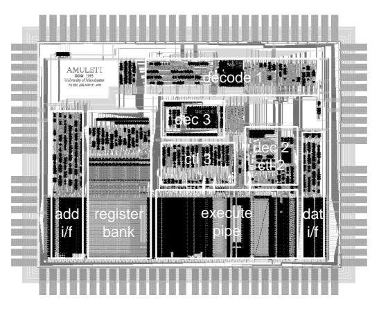
Figure 10. The asynchronous ARM chip
