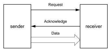
Figure 1. A two-phase bundled data interface
