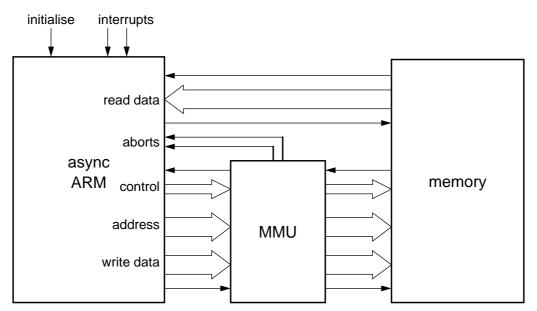
Figure 2. The processor interface
