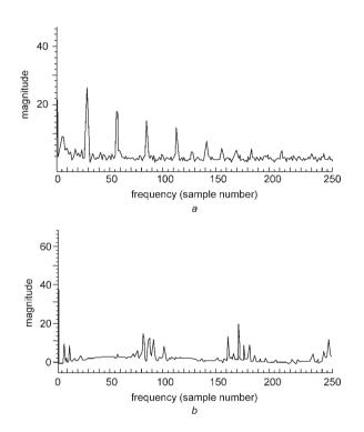
**Fig. 4** *FFT of current consumption in synchronous and desynchronised DLX*
