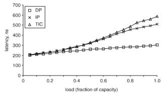
Fig. 13 Latency of IP, DP and TIC masters
