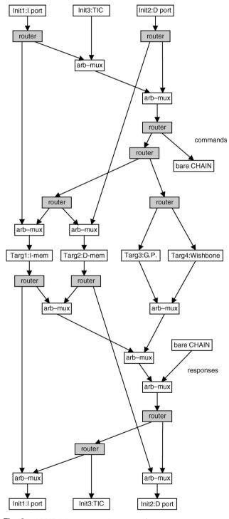
Fig. 9 ASPIDA interconnection network
