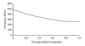
**Fig. 10** Impact of TIC load on throughput of IP Note that TIC has same impact on throughput of DP master
