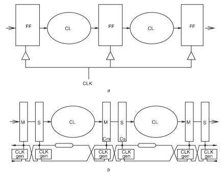
Fig. 2 Synchronous and desynchronised pipelined circuit
