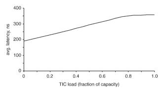
Fig. 11 Latency of IP master against TIC load
