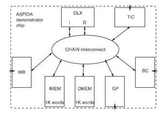
Fig. 8 Top-level block diagram of ASPIDA demonstrator chip
