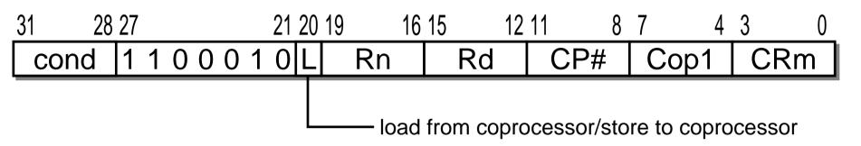
O move a 64-bit value between the coprocessor and ARM
