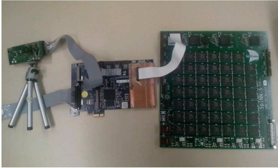
(a) Picture of the neuromorphic visual processing platform. From left to right: a silicon retina, an FPGA board which converts AER packets to SpiNNaker format, and a 48-node SpiNNaker system.
