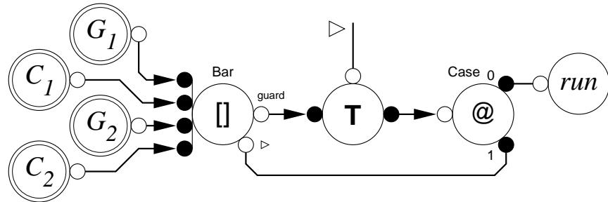
**Figure 5.1.** An *if* command implemented using Case
