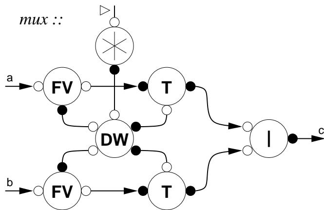
**Figure 3.1.** *mux* implementation in handshake components
