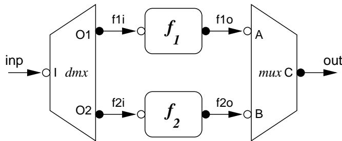
**Figure 3.5.** Handshake circuit implementation of the example pipeline
