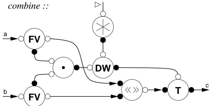
**Figure 3.2.** `combine` implementation in handshake components
