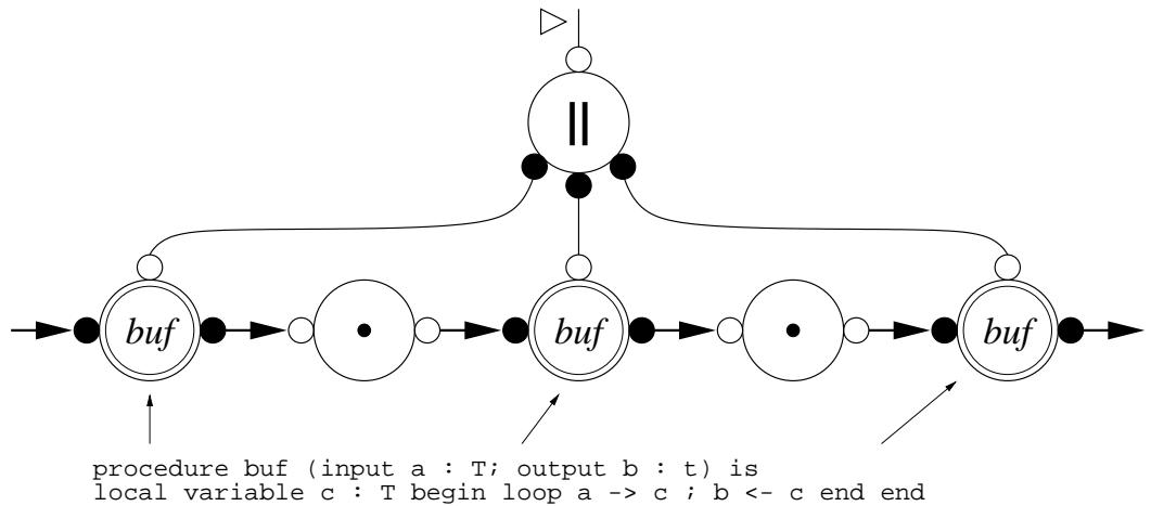
**Figure 2.1.** A Passivator-connected pipeline of buffer elements
