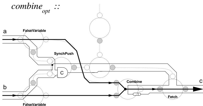
**Figure 5.9.** Gate level implementation of *combine* – after gate level optimisation
