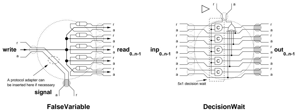
**Figure 5.3.** Gate level implementations of FalseVariable and DecisionWait
