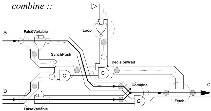
**Figure 5.8.** Gate level implementation of *combine* – before gate level optimisation
