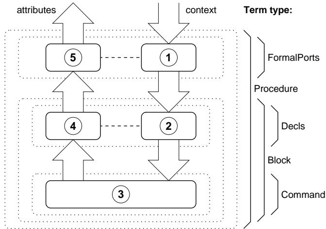
**Figure 4.2.** Procedure compilation in the balsa-c attribute grammar evaluator
