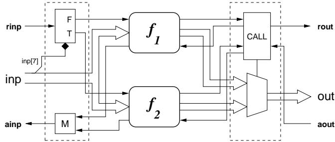
**Figure 3.4.** Micropipeline implementation of the example pipeline
