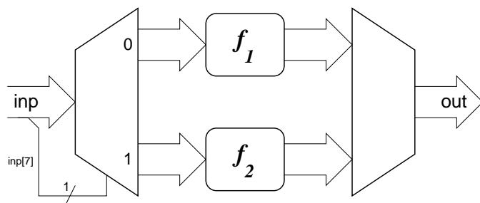
**Figure 3.3.** An example unbuffered pipeline
