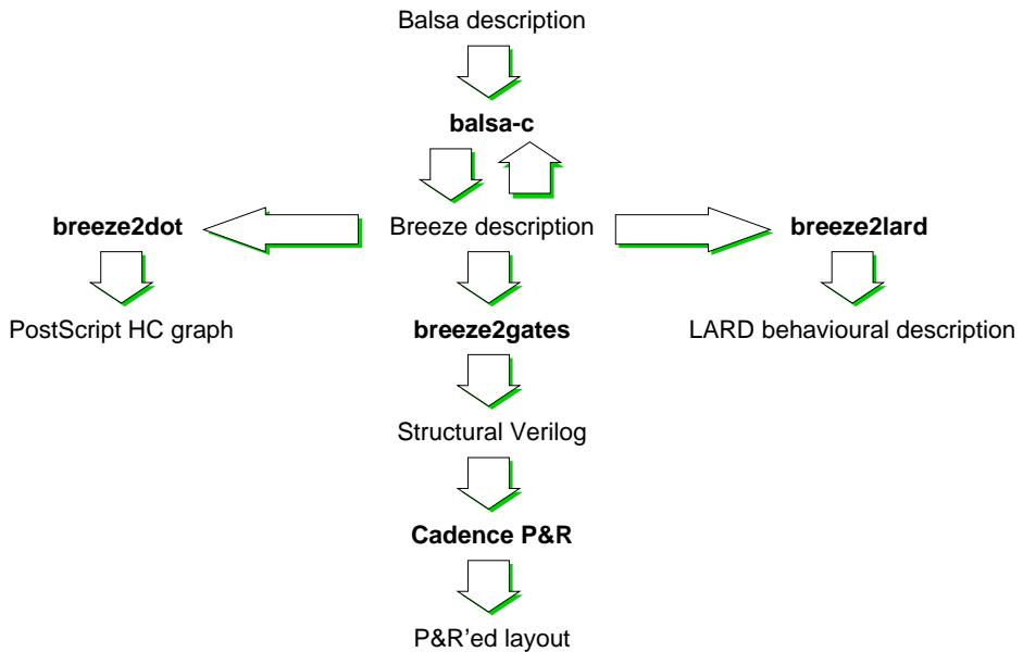
**Figure 4.1.** Balsa design flow
