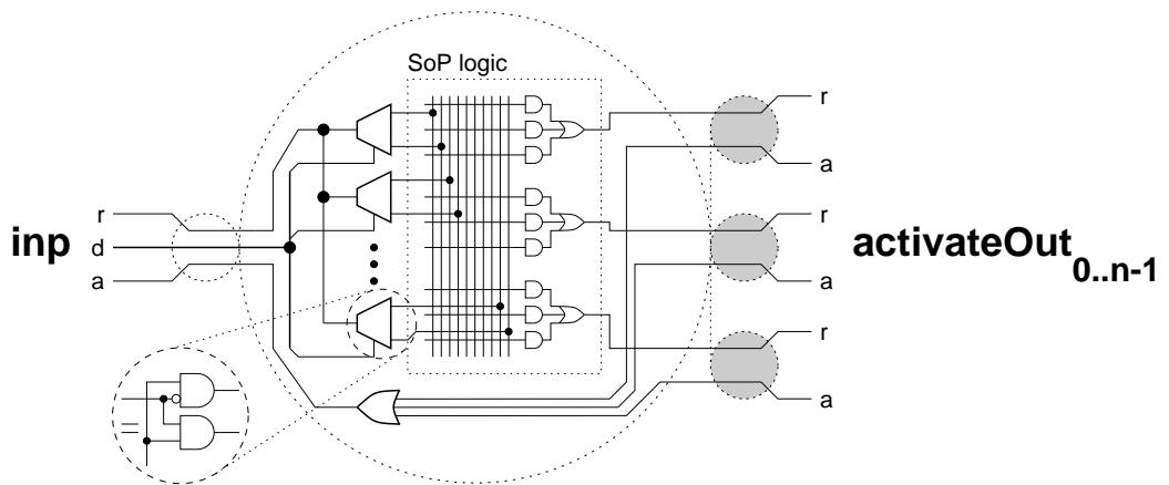
**Figure 5.6.** The Balsa Case component's implementation
