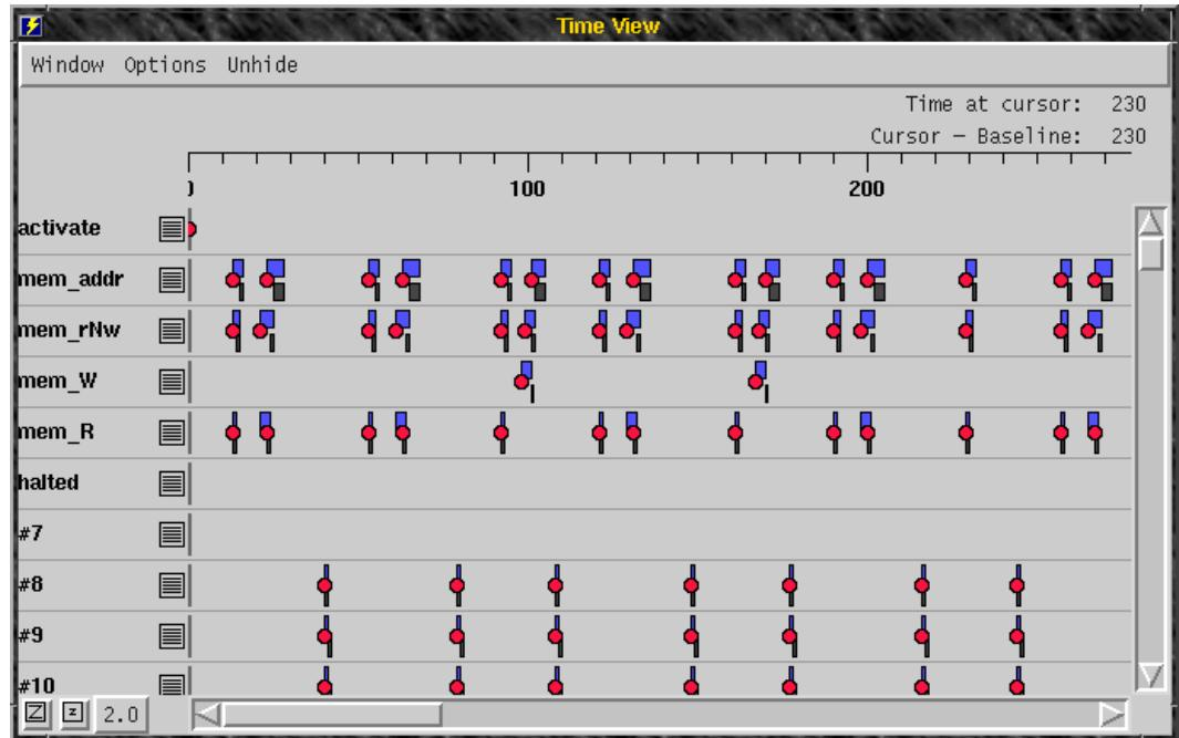
**Figure 6.2.** SSEM test program running in LARD
