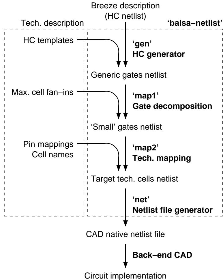
**Figure 4.2.** Balsa back-end design flow
