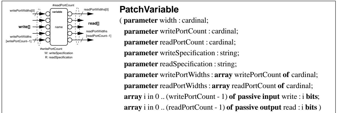
**Figure 5.4.** Generalised variable handshake component – PatchVariable
