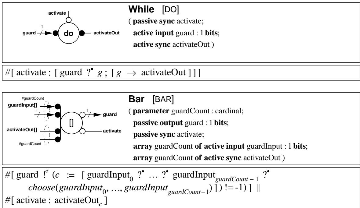
Figure 3.4. While and Bar handshake components
