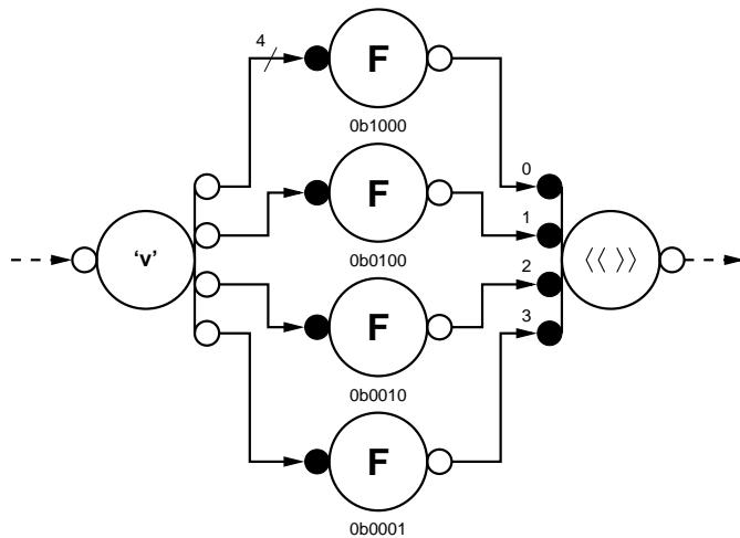
**Figure 5.3.** 4b bit reverser handshake circuit
