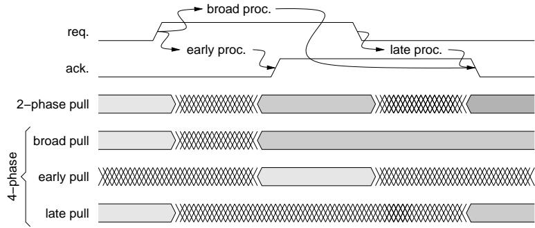
**Figure 1.3.** 2/4-phase pull handshaking
