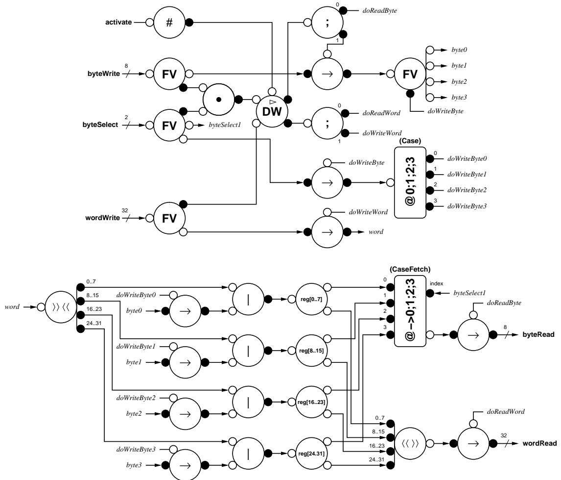
**Figure 5.5.** WordReg implementation using Variable components
