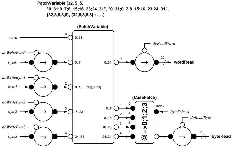
**Figure 5.6.** WordReg implementation using a PatchVariable component
