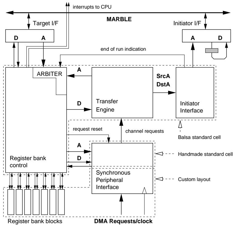
**Figure 6.3.** DMA controller structure
