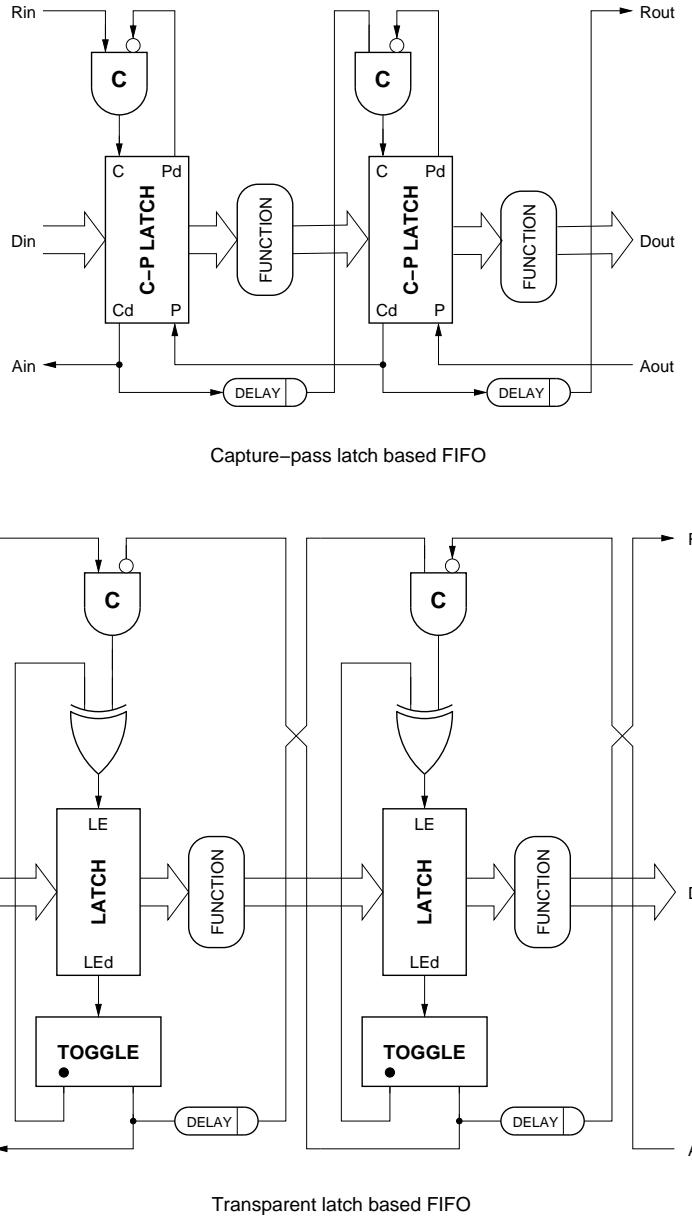
**Figure 2.4.** FIFOs with capture-pass and transparent latches
