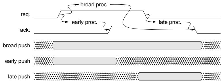
**Figure 1.2.** 4-phase push handshaking
