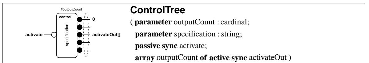
**Figure 5.7.** Generalised control tree handshake component – ControlTree
