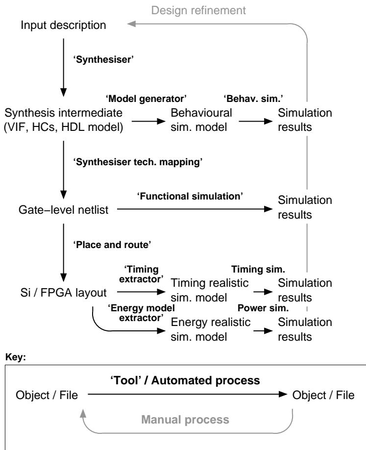
**Figure 2.1.** Typical synthesis design flow
