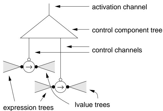
**Figure 4.4.** Control tree structure in handshake circuits
