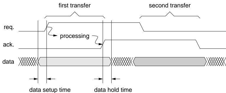
**Figure 1.1.** 2-phase handshaking
