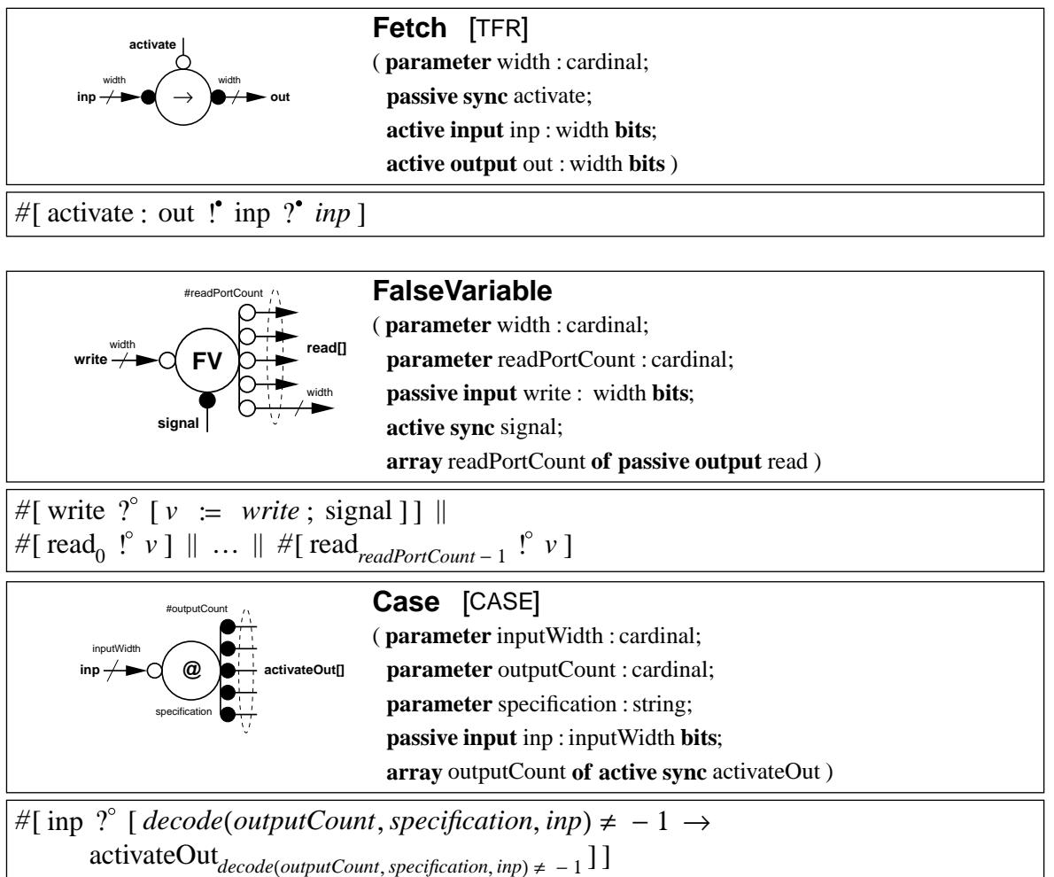
**Figure 3.5.** Fetch, FalseVariable and Case handshake components
