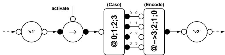
**Figure 5.11.** 2b complement operation – using Encode
