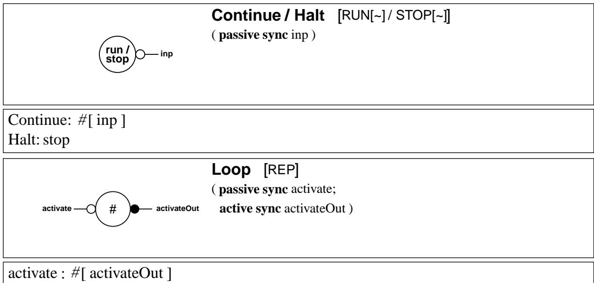
**Figure 3.2.** Continue, Halt and Loop handshake components
