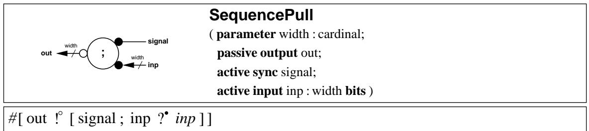
**Figure 4.6.** SequencePull handshake component
