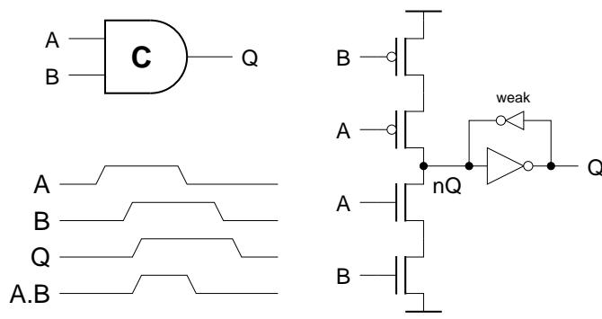
**Figure 1.5.** The Muller C-element
