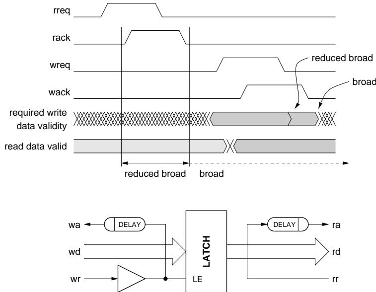
**Figure 1.4.** A latch using reduced broad push and pull protocols
