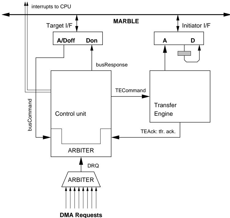
**Figure 7.2.** Simplified DMA controller structure
