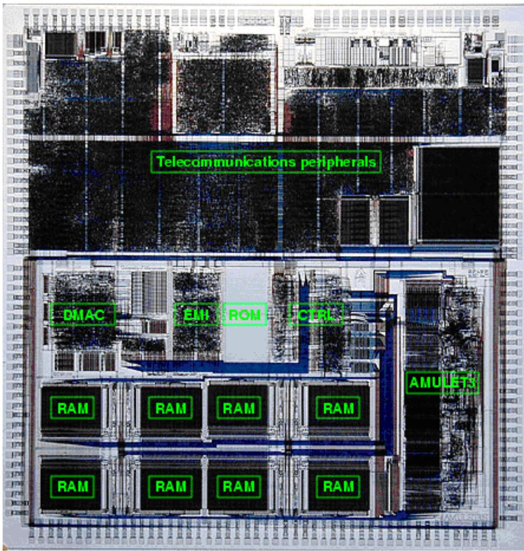
**Figure 6.2.** DRACO communications IC (AMULET3i is the lower half of this IC)
