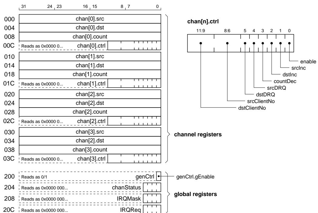
Figure 7.1. Simplified DMA controller programmer’s model
