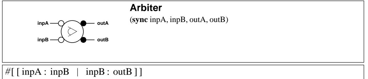
**Figure 3.14.** Arbiter handshake component
