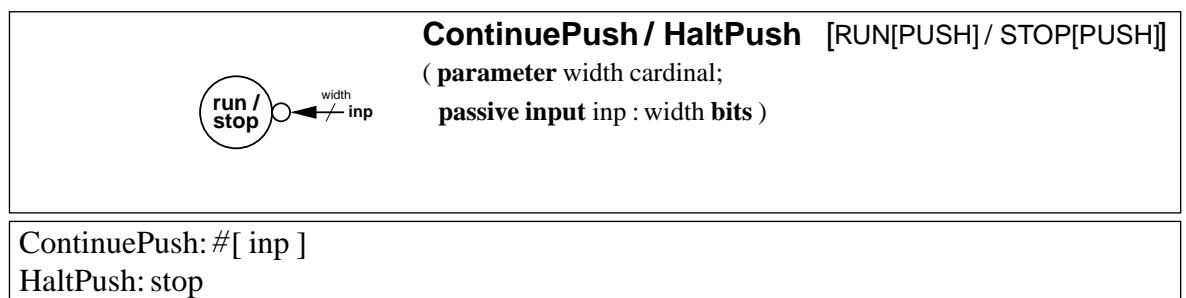
**Figure 3.9.** ContinuePush and HaltPush handshake components
