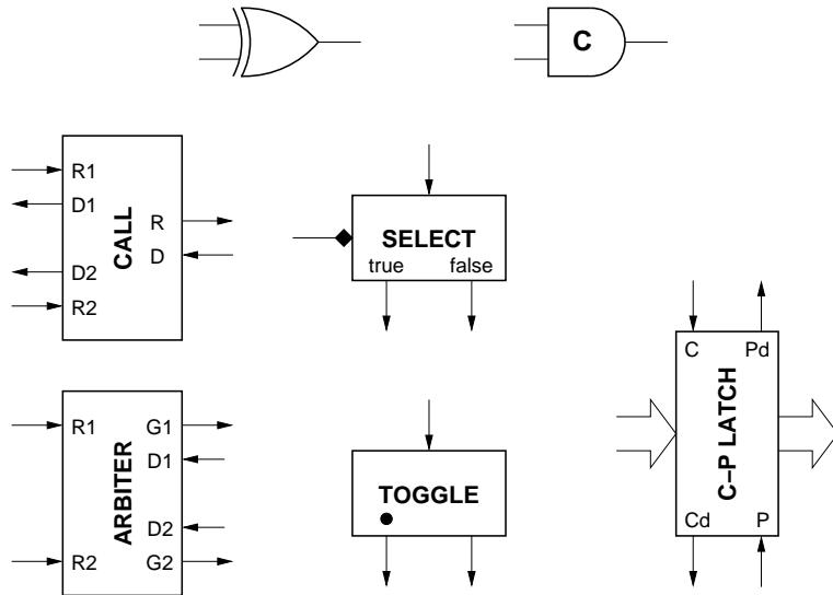
**Figure 2.2.** Micropipeline elements
