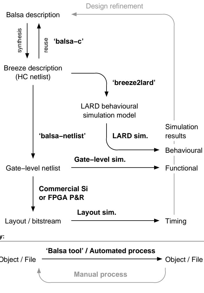
**Figure 4.1.** Balsa design flow
