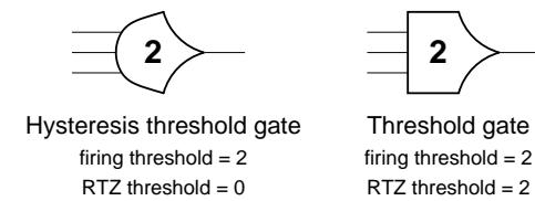
**Figure 2.7.** NCL threshold gates
