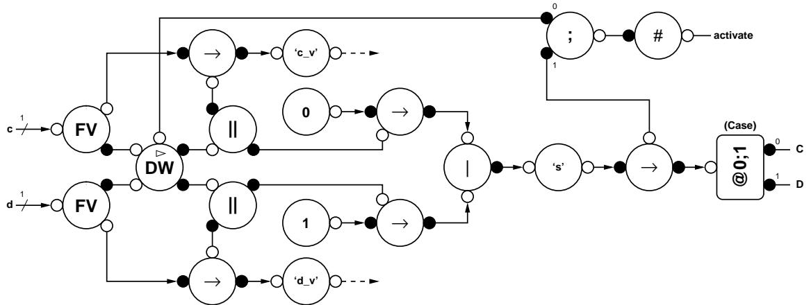
**Figure 5.2.** Tangram-style select handshake circuit
