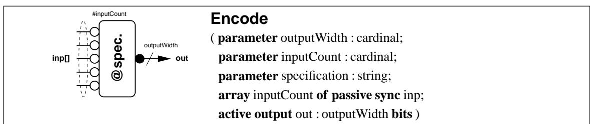
**Figure 5.9.** Encode handshake component
