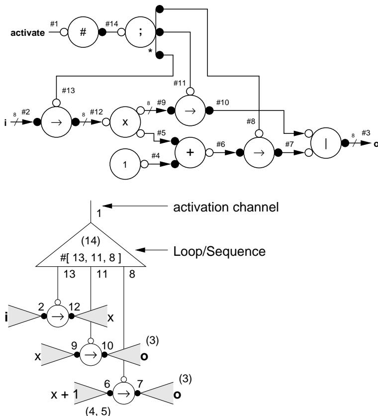
**Figure 4.5.** A simple buffer example: handshake circuit and activation tree
