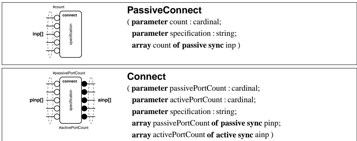
**Figure 5.8.** Generalised sync interconnect – `PassiveConnect`, `Connect`
