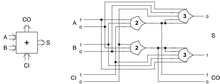
**Figure 2.8.** NCL hysteresis threshold gate adder
