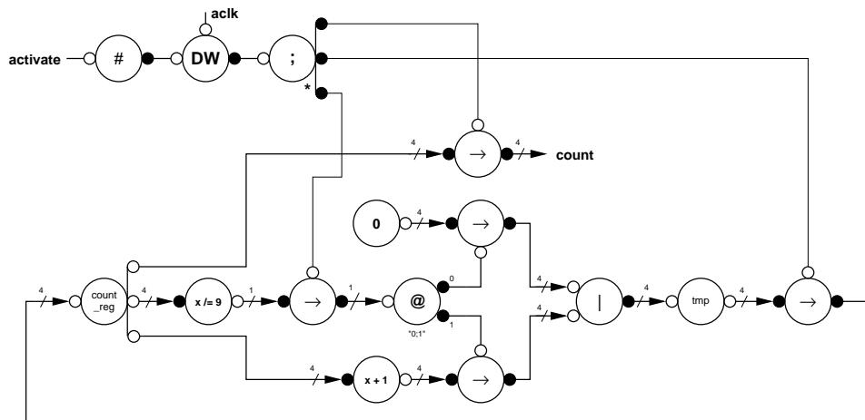
**Figure 3.1.** A simple handshake circuit (a modulo-10 counter)
