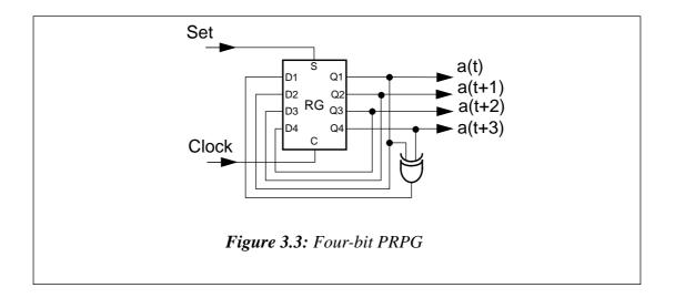
terns generated by an LFSR is deterministic, a non-homogeneous Bernouilli process can be used for simulation. This is called pseudo-random pattern generation [24].
