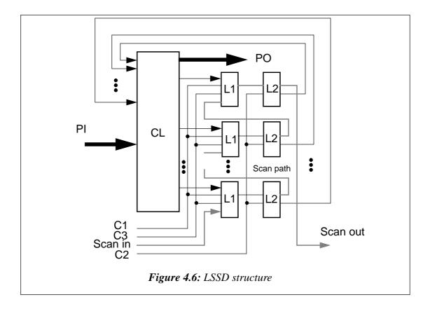
The basic algorithm for testing with the LSSD structure shown in Figure 4.6 can be written as follows:
