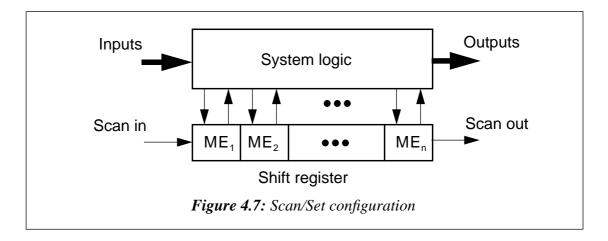
ters of the circuit can be obtained. The internal nodes of the circuit which are to be connected to the shift register are derived from the results of testability analysis programs [14,28].
