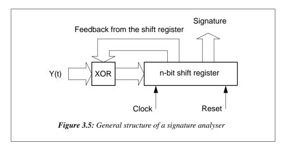
is the residue of the division. In other words, the residue of dividing the input polynomial describing the data flow into the primitive polynomial is the signature.
