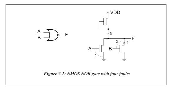
level. Theoretically, for any circuit the total number of all possible faulty circuits with multiple stuck-at faults can be estimated as  $3^n - 1$ , where n is the number of nodes in the circuit. In practice, only single stuck faults are considered in order to eliminate an incredibly large number of faulty VLSI circuits.
