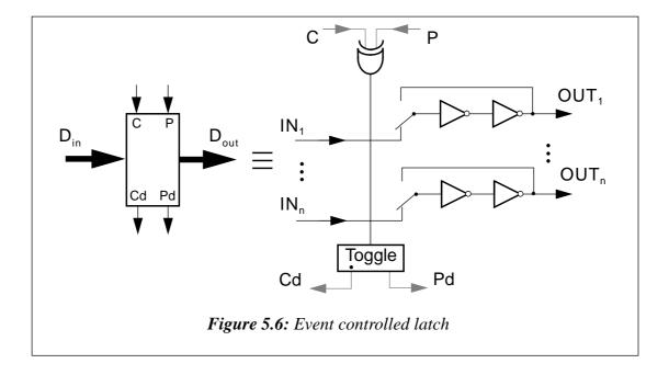
Single stuck-at faults. Any stuck-at fault on the inputs or outputs of the latch is equivalent to the appropriate fault in the combinational logic. A stuck-at fault on the control (dotted) lines of the latch (Figure 5.6) prevents the generation of any events in the latch. This causes the micropipeline to halt. The absence of activity in the micropipeline can easily be identified and, hence, there is no need for test generation for such faults.
