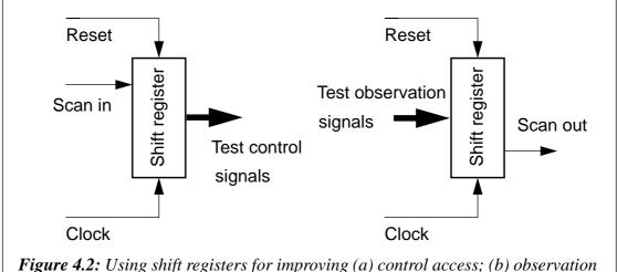
Figure 4.2: Using shift registers for improving (a) control access; (b) observation access
