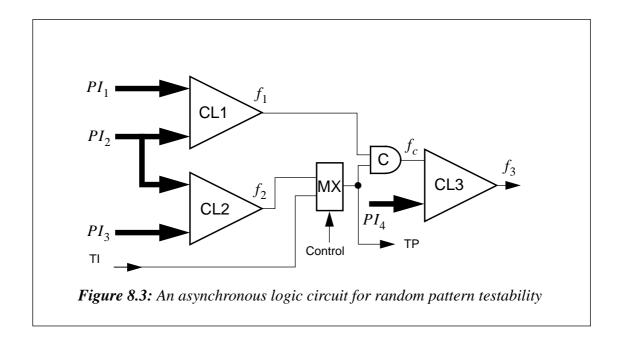
In *the normal operation mode* the control signal of the multiplexer is set to connect the output of CL2 with the input of the Muller-C element. In this case additional input TI and output TP are not used.
