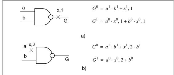
Figure 5.3: Equations for handling faults in a NAND circuit for the case of a) stuck-at-0 fault at the output; b) stuck-at-1 fault at input a
