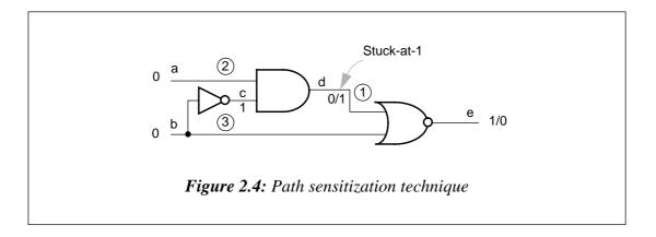
through the NOR gate to the output e. Therefore, the result of the justification step can be propagated only if a logical 0 is set on line a. The effect of the propagation process (step 3) is to move the fault effect through a sensitized path to an output of the circuit.
