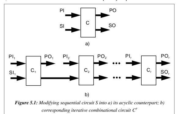
As a result, the test consists of an ordered set of r input patterns applied to the primary inputs PI of S. After that the behaviour of S is simulated while applying the derived set of patterns. If during the simulation no races or hazards are registered in S, then the test is accepted as a test for fault F in S.
