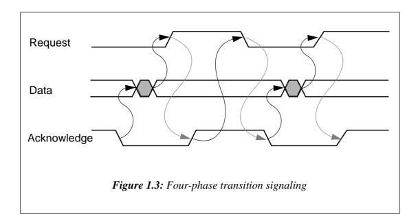
two-phase bundled data convention the interpretation of transitions requires more control logic than four-phase signalling requires.
