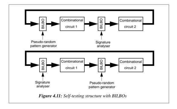
test. The simlex method is more efficient for self-testing pipelined structures but it has considerable drawbacks for circuits in which the inputs to one block are formed from the outputs of many other blocks. In such cases duplex methods must be used where each functional block has its own PRPG and signature analyser.
