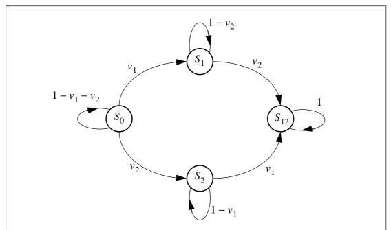
Figure 7.3: The Markov chain describing the process of the appearance of two different random patterns
