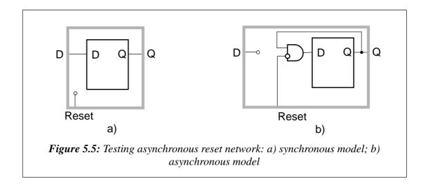
programs is proposed to generate tests for asynchronous set/reset circuits. The model shown in Figure 5.5a is used to simulate the synchronous test procedure. For simulating asynchronous testing, the model shown in Figure 5.5b is used.
