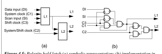
Figure 4.5: Polarity hold latch (a) symbolic representation; (b) implementation in NAND gates
