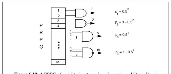
Figure 6.10: A PRPG of weighted patterns based on using additional logic
