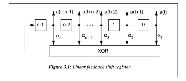
Figure 3.1 shows the general structure of an LFSR. Symbol  $\alpha_i$  indicates the presence  $(\alpha_i = 1)$  or absence  $(\alpha_i = 0)$  of a feedback connection from the output of the *i*th stage to the XOR network. Sometimes the coefficients  $\alpha_i$  are called "taps" since they determine the structure of the LFSR.
