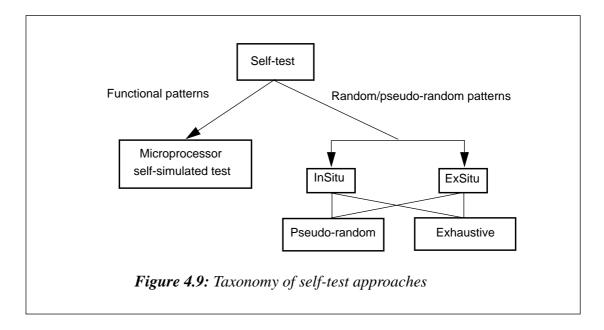
difference between these two approaches is that InSitu self-test uses system registers to generate and compact test data whereas the ExSitu structure uses registers external to the system function to generate tests and analyse the responses of the circuit.
