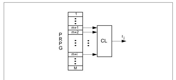
Figure 6.7: A general structure of a PRPG with given signal probabilities on its outputs
