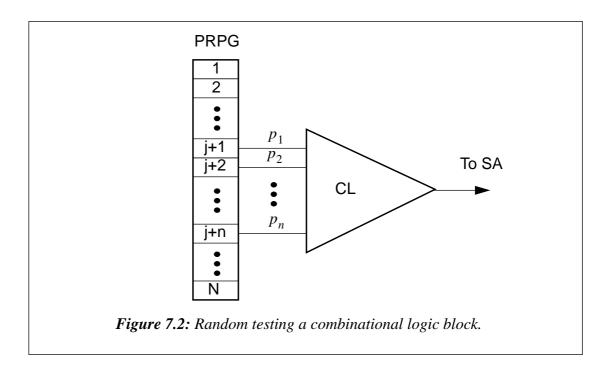
one pattern from the set  $Q_m$  will not be applied to the inputs of the combinational logic during the test. The test length,  $T_m$ , is the total number of test patterns applied to the inputs of the circuit.
