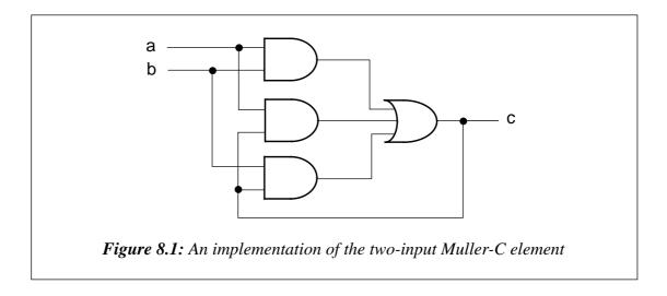
2) to calculate the probabilities of each cube of F and find the sum of these probabilities [61-63]. In the case of the two-input Muller-C element, its Boolean function (20) can be written as:
