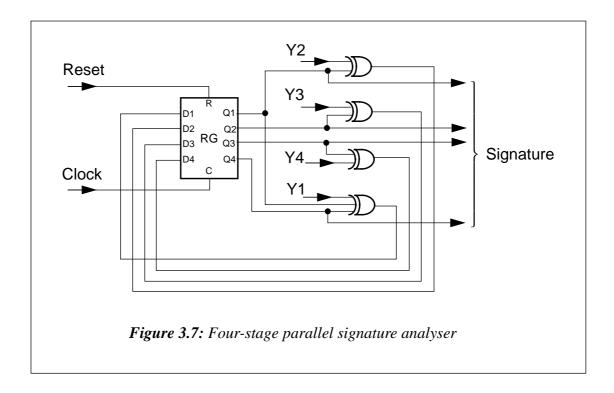
In practice, two basic kinds of signature analysers are used: serial and parallel signature analysers [28]. A four-stage serial signature analyser and four-stage parallel signature analyser are shown in Figure 3.6 and Figure 3.7 respectively. A serial signature analyser treats only one response bit at every clock whereas a parallel signature analyser compacts responses from the outputs of multiple networks under test.
