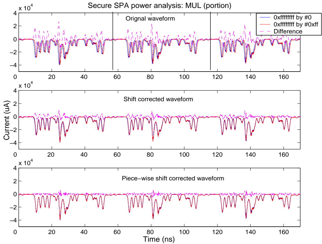
Figure 4.5 An example of waveform shift correction
