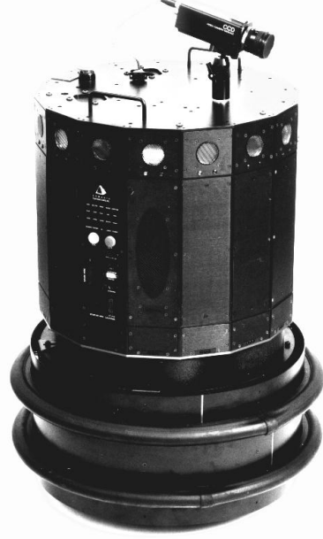
Figure 2: The Nomad 200 mobile robot FortyTwo used in the experiments reported here.
