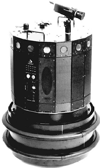
Fig. 1. *The Manchester 'FortyTwo'*. Exploration was carried out using the translational and rotational motors located in the base of the robot. A separate behaviour was used to rotate the turret at small speeds towards "North" as indicated by a compass (see Section 5 for full details).
