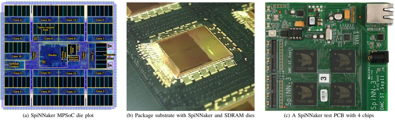
Fig. 4. SpiNNaker chip and a 3<sup>rd</sup> generation SpiNNaker PCB
