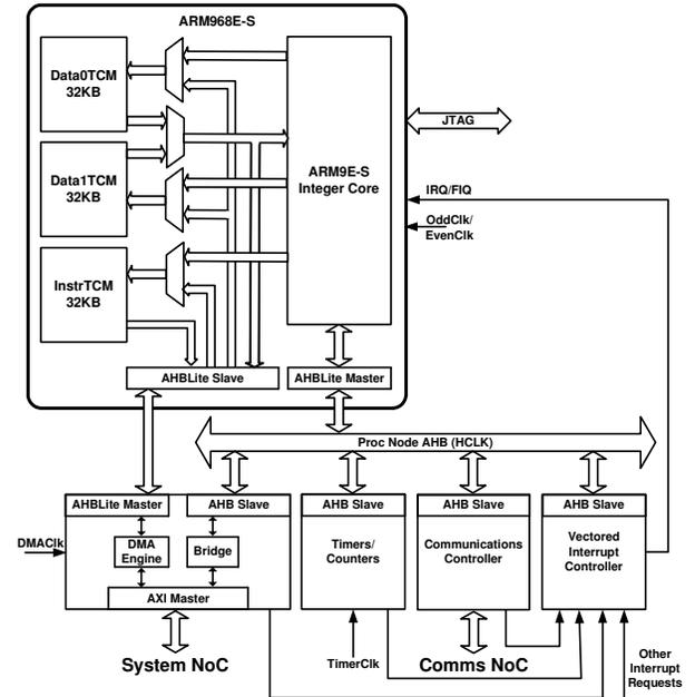
Fig. 3. Details of a SpiNNaker Processor Node
