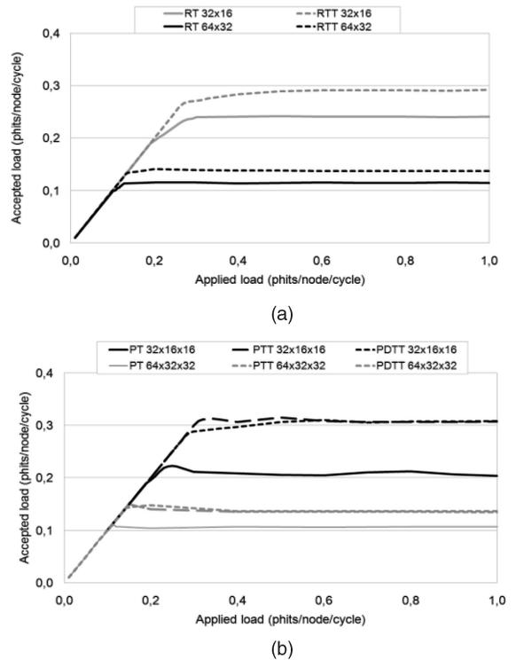
Fig. 11. Throughput under HR traffic for (a) 2D and (b) 3D networks.
