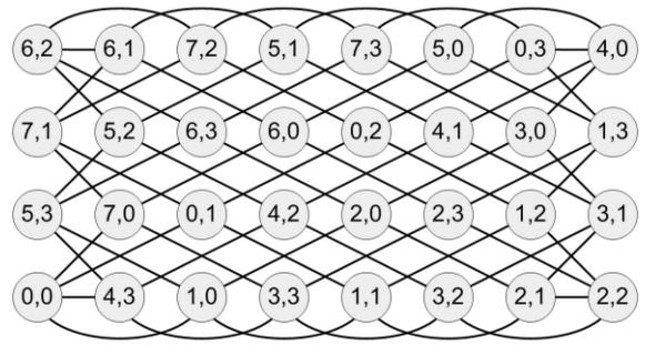
Fig. 15. Trellis folded RTT of size  $8 \times 4$ .
