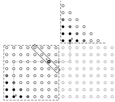
Fig. 6. Path between two nodes in an RTT of size  $16 \times 8$ . Vivid circles on the down left side represent nodes in one-half of the network, while dashed square represents the bisection. Pale circles on the down right side represent nodes in the other half of the network. For the sake of clarity, a fragment of a replica tile is showed in the upright side. Note that the shortest path from A to B crosses the bisection twice.
