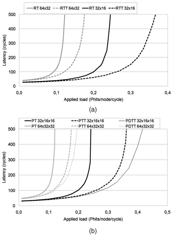
Fig. 9. Average latency under random uniform traffic for (a) 2D and (b) 3D networks.
