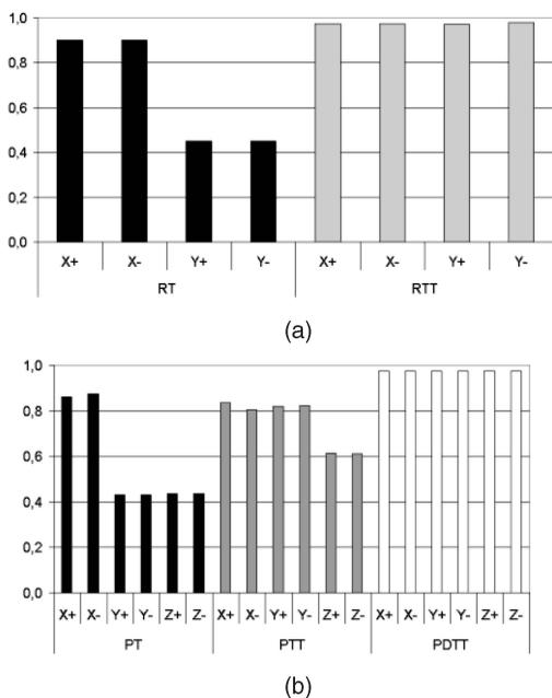
Fig. 10. Average link utilization under random uniform traffic for (a) 2D and (b) 3D networks, with the network saturated.
