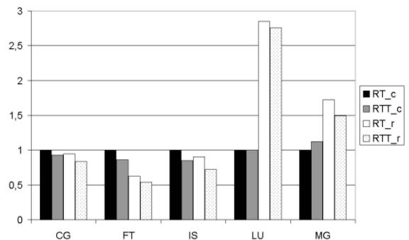
Fig. 14. Total time required to fully inject and deliver the workload with real applications on a  $16 \times 8$  network.
