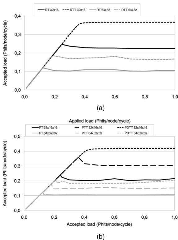
Fig. 8. Throughput for (a) 2D and (b) 3D networks under random uniform traffic.
