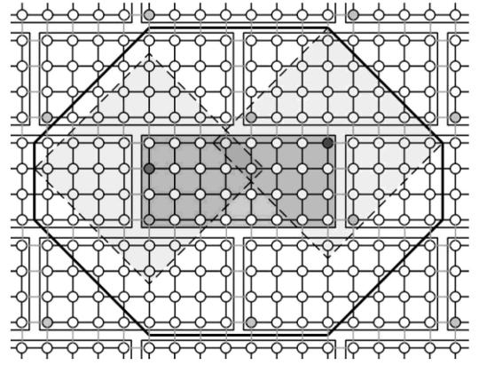
Fig. 5. Possible paths departing from an  $8 \times 4$  RTT. The original tile (corresponding to nodes 1-32) is shadowed and centered.
