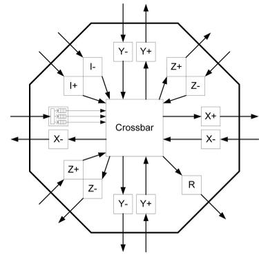
Fig. 7. Model of the simulated routers, with a detailed view of the X+ input port showing the three virtual channels that share this link. The 2D case would not include ports and links for the Z axis.
