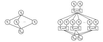
Fig. 6 Dependency graph for regular dataflow execution (left graph) and double execution (right graph).
