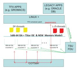
Fig. 7 Overall picture of the "simulator illusion". A number n of VCPUs can be used as "workers" or "x86-64 crunchers" or "auxiliary cores"; a generic kth VCPU can be used as service core. L- and S-threads represent legacy and system Threads, that our system is able to execute.
