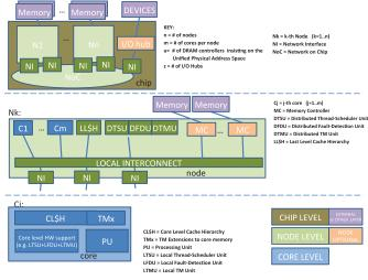
Fig. 5 TERAFLUX Architecture Template.
