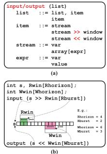
Fig. 4 Syntax for input and output clauses (a) and illustration of stream access through windows (b).
