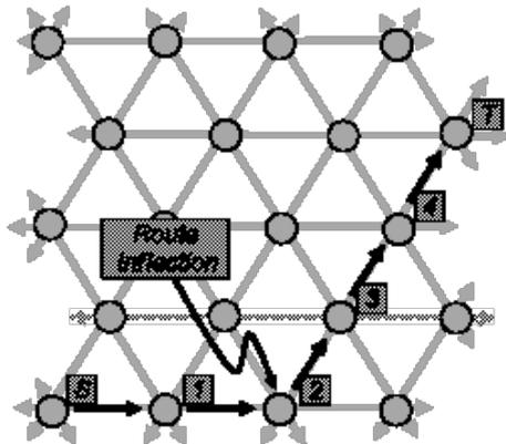
**Figure 3: Chip level SpiNNaker interconnect**
