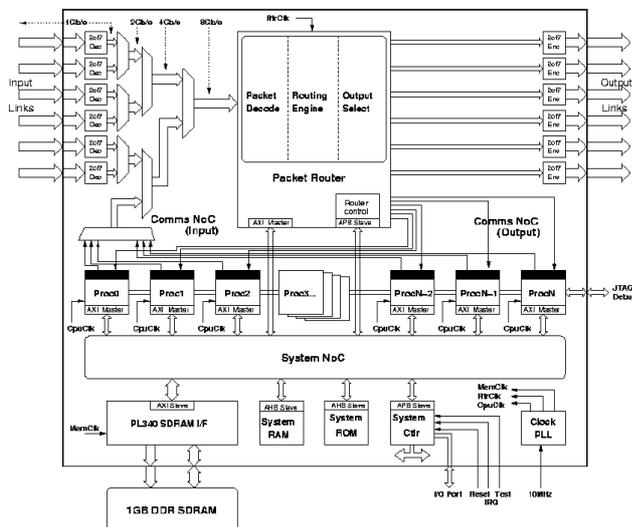
**Figure 1:** A single SpiNNaker node internals
