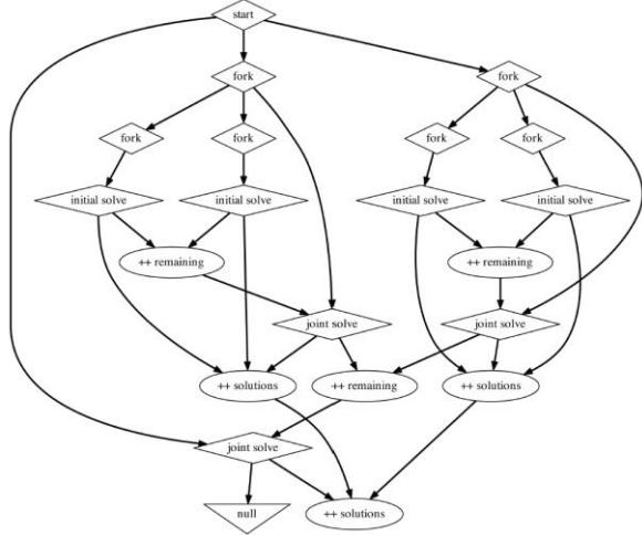
Fig. 3 An instance of a dataflow graph for a circuit routing algorithm.
